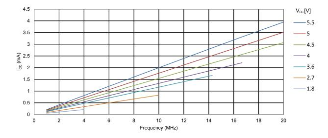
Figure 34-54. ATmega328PB: Reset Supply Current vs. Vcc (Excluding current through Reset Pullup)
