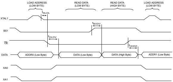
Note: The timing requirements shown in Parallel Programming Characteristics (i.e., t<sub>DVXH</sub>, t<sub>XHXL</sub>, and  $t_{\text{XLDX}}$ ) also apply to reading operation.
