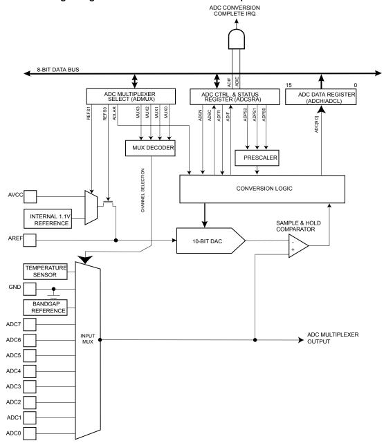
Figure 28-1. Analog to Digital Converter Block Schematic Operation
