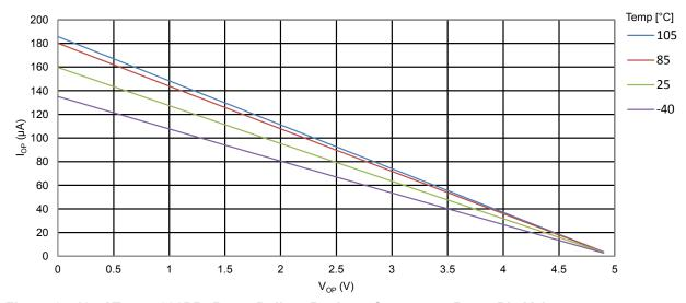
Figure 34-19. ATmega328PB: Reset Pull-up Resistor Current vs. Reset Pin Voltage ( $V_{CC} = 1.8V$ )
