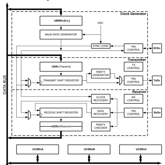
Figure 24-1. USART Block Diagram
