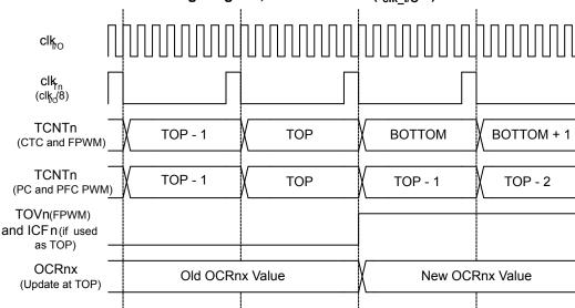
Figure 19-12. Timer/Counter Timing Diagram, with Prescaler (f<sub>clk I/O</sub>/8)
