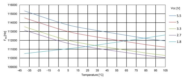
Figure 34-42. ATmega328PB: Watchdog Oscillator Frequency vs. V<sub>CC</sub>
