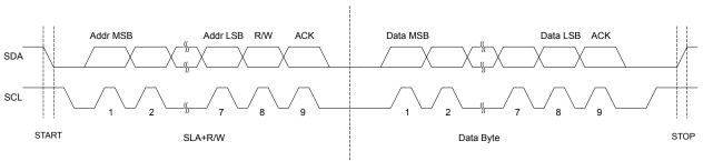
Figure 26-6. Typical Data Transmission
