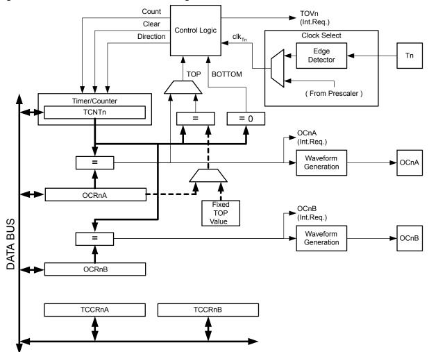
Figure 18-1. 8-bit Timer/Counter Block Diagram
