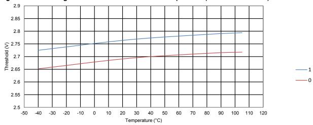
Figure 34-34. ATmega328PB: BOD Thresholds vs. Temperature (BODLEVEL is 4.3V)
