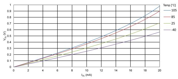
Figure 34-23. ATmega328PB: I/O Pin Output Voltage vs. Sink Current (V<sub>CC</sub> = 5V)
