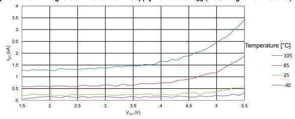
Figure 34-14. ATmega328PB: Power-Down Supply Current vs. V<sub>CC</sub> (Watchdog Timer Enabled)
