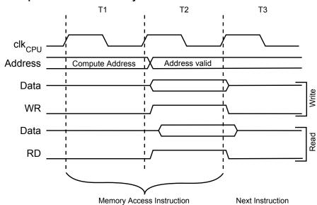
Figure 10-3. On-chip Data SRAM Access Cycles
