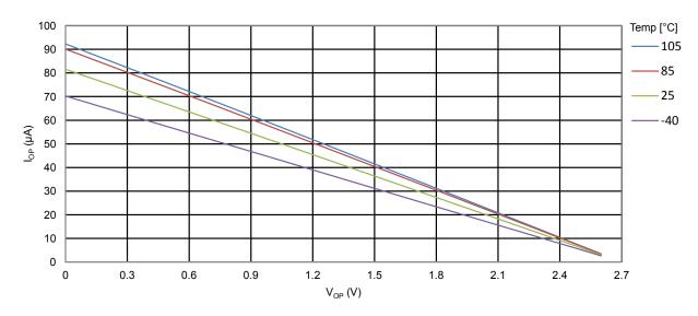
Figure 34-18. ATmega328PB: I/O Pin Pull-up Resistor Current vs. Input Voltage (V<sub>CC</sub> = 5V)
