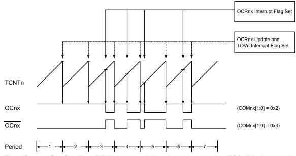
The Timer/Counter Overflow Flag (TOV2) is set each time the counter reaches TOP. If the interrupt is enabled, the interrupt handler routine can be used for updating the compare value.
