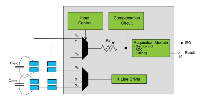
Figure 29-2. PTC Block Diagram Self-Capacitance
