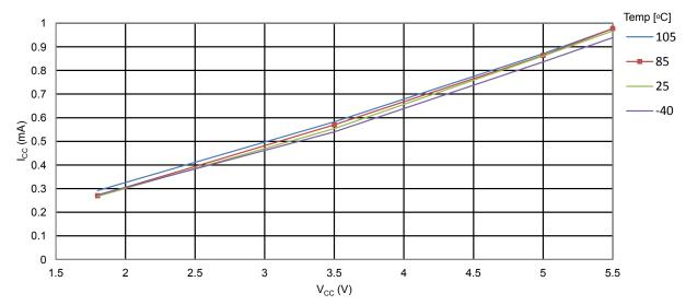
Figure 34-5. ATmega328PB: Active Supply Current vs. V<sub>CC</sub> (Internal RC Oscillator, 8MHz)
