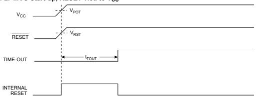
Figure 14-3. MCU Start-up, RESET Extended Externally
