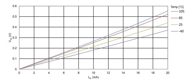
Figure 34-24. ATmega328PB: I/O Pin Output Voltage vs. Source Current (V<sub>CC</sub> = 3V)
