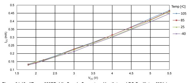
Figure 34-12. ATmega328PB: Idle Supply Current vs. V<sub>CC</sub> (Internal RC Oscillator, 8MHz)
