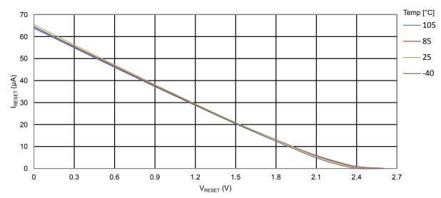
Figure 34-21. ATmega328PB: Reset Pull-up Resistor Current vs. Reset Pin Voltage (V<sub>CC</sub> = 5V)
