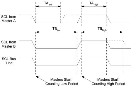
Figure 26-7. SCL Synchronization Between Multiple Masters
