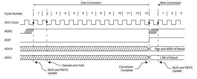
Figure 28-6. ADC Timing Diagram, Auto Triggered Conversion
