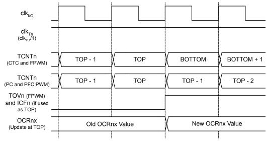
**Note:** The "n" in the register and bit names indicates the device number (n = 1, 3, 4 for Timer/Counter 1, 3, 4), and the "x" indicates Output Compare unit (A/B).
