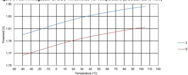
Figure 34-33. ATmega328PB: BOD Thresholds vs. Temperature (BODLEVEL is 2.7V)
