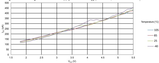
Figure 34-7. ATmega328PB: Active Supply Current vs. V<sub>CC</sub> (With ADC, No conversion)
