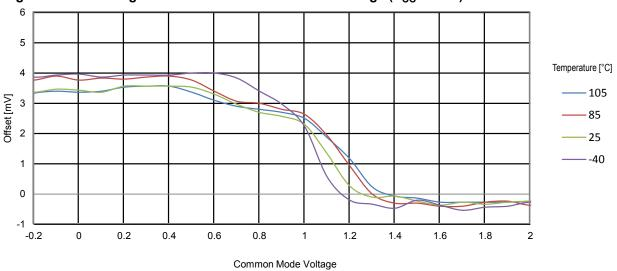
Figure 34-39. ATmega328PB AC Offset vs. Common Voltage (V<sub>CC</sub> = 3.0V)
