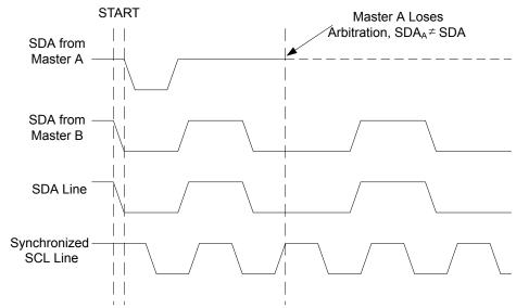
Figure 26-8. Arbitration Between Two Masters
