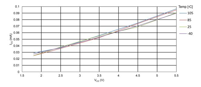
Figure 34-4. ATmega328PB: Active Supply Current vs. V<sub>CC</sub> (Internal RC Oscillator, 1MHz)
