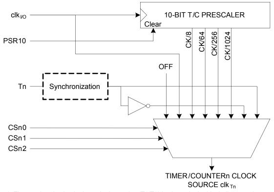
**Note:** 1. The synchronization logic on the input pins (T1/T0) is shown in the block diagram above.
