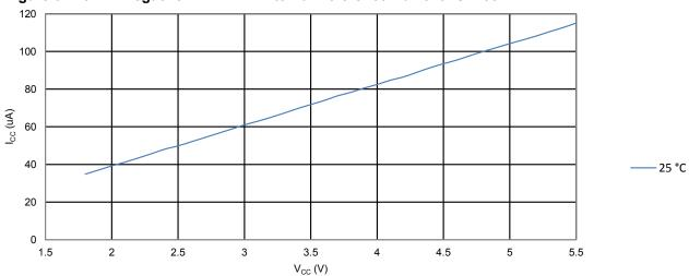
Figure 34-50. ATmega328PB: Brownout Detector Current vs. Vcc
