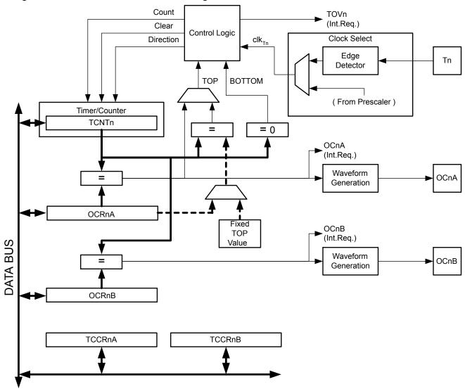
Figure 21-1. 8-bit Timer/Counter Block Diagram
