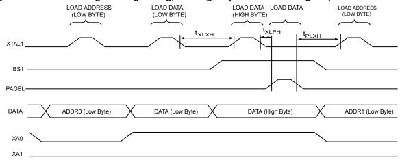
**Note:** The timing requirements shown in Parallel Programming Characteristics (i.e.,  $t_{DVXH}$ ,  $t_{XHXL}$ , and  $t_{XLDX}$ ) also apply to loading operation
