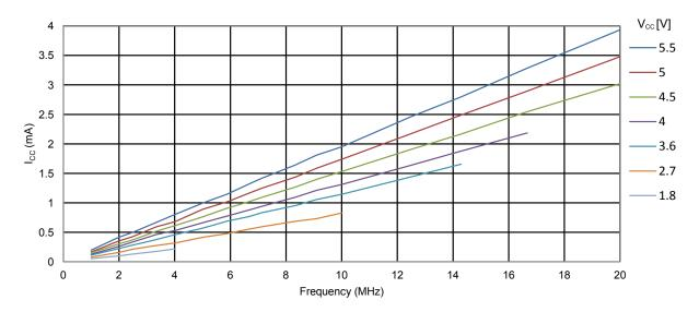
Figure 34-10. ATmega328PB: Idle Supply Current vs. V<sub>CC</sub> (Internal RC Oscillator, 128kHz)
