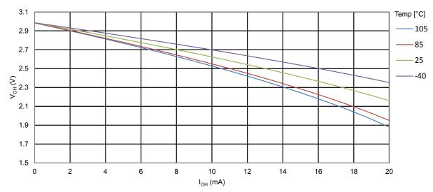
Figure 34-25. ATmega328PB I/O Pin Output Voltage vs. Source Current ( $V_{CC} = 5V$ )
