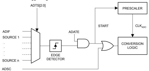
Using the ADC Interrupt Flag as a trigger source makes the ADC start a new conversion as soon as the ongoing conversion has finished. The ADC then operates in Free Running mode, constantly sampling and updating the ADC Data Register. The first conversion must be started by writing a '1' to
