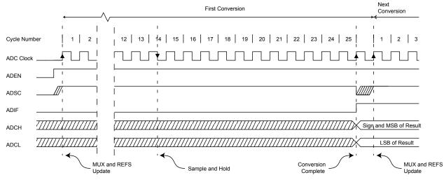
Figure 28-5. ADC Timing Diagram, Single Conversion
