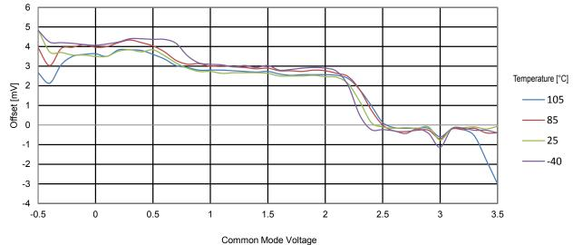
Figure 34-40. ATmega328PB AC Offset vs. Common Voltage (V<sub>CC</sub> = 5.0V)
