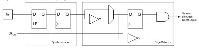
The synchronization and edge detector logic introduces a delay of 2.5 to 3.5 system clock cycles from an edge has been applied to the T1/T0 pin to the counter is updated.
