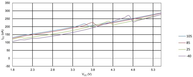
Figure 34-48. ATmega328PB: Analog Comparator Current vs. Vcc
