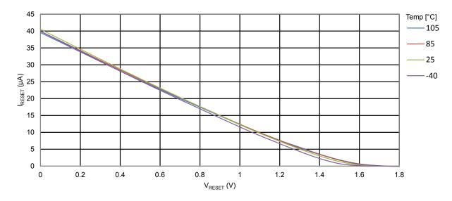
Figure 34-20. ATmega328PB: Reset Pull-up Resistor Current vs. Reset Pin Voltage  $(V_{CC} = 2.7V)$
