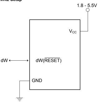
The debugWIRE Setup shows the schematic of a target MCU, with debugWIRE enabled, and the emulator connector. The system clock is not affected by debugWIRE and will always be the clock source selected by the CKSEL Fuses.
