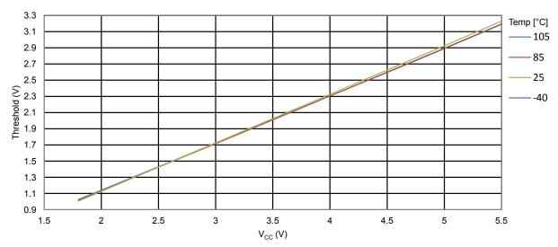
Figure 34-27. ATmega328PB I/O Pin Input Threshold Voltage vs.  $V_{CC}$  ( $V_{IL}$ , I/O Pin read as '0')
