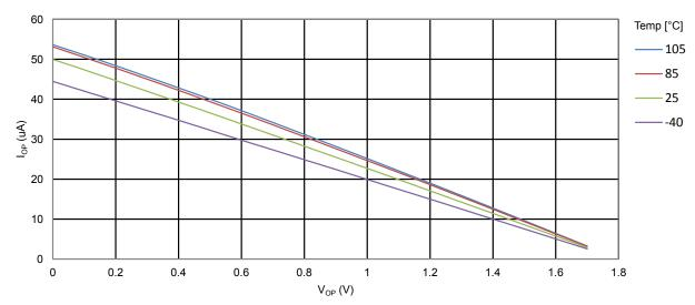
Figure 34-17. ATmega328PB: I/O Pin Pull-up Resistor Current vs. Input Voltage (V<sub>CC</sub> = 2.7V)
