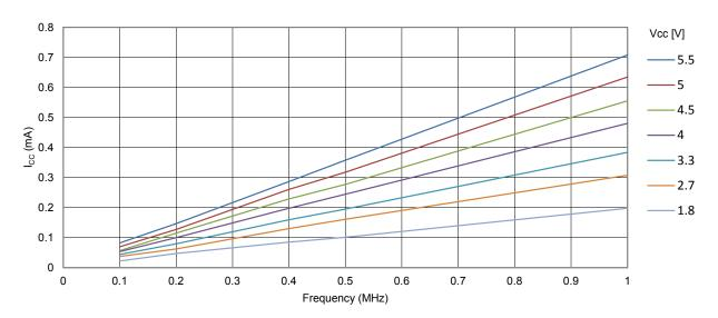
Figure 34-2. ATmega328PB: Active Supply Current vs. Frequency (1-20MHz)
