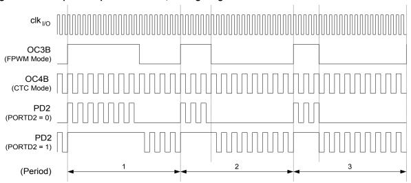
Figure 22-3. Output Compare Modulator, Timing Diagram
