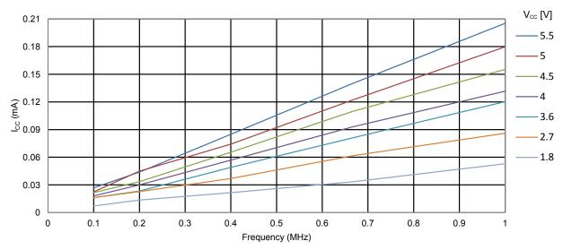
Figure 34-9. ATmega328PB: Idle Supply Current vs. Frequency (1-20MHz)
