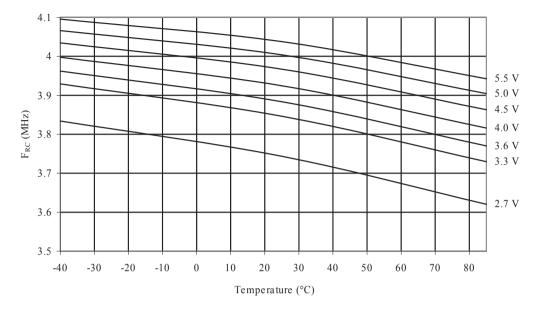
Figure 34-47 Calibrated 4 MHz RC Oscillator Frequency vs. V<sub>CC</sub>
