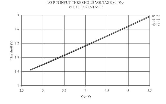
Figure 34-30 I/O Pin Input Threshold Voltage vs. V<sub>CC</sub> (VIH, I/O Pin Read as '1')
