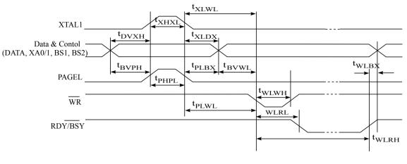
Figure 32-5 Parallel Programming Timing, Loading Sequence with Timing Requirements<sup>(1)</sup>
