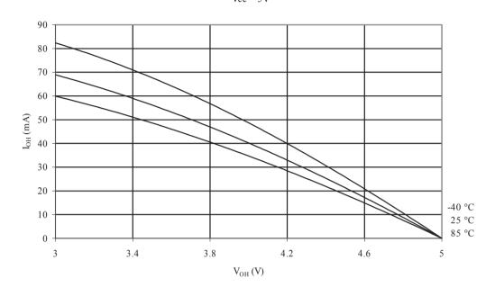
I/O PIN SOURCE CURRENT vs. OUTPUT VOLTAGE Vcc = 5V
