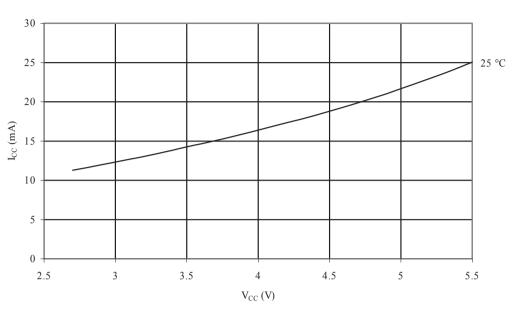
IDLE SUPPLY CURRENT vs. V<sub>CC</sub> EXTERNAL RC OSCILLATOR, 32 kHz
