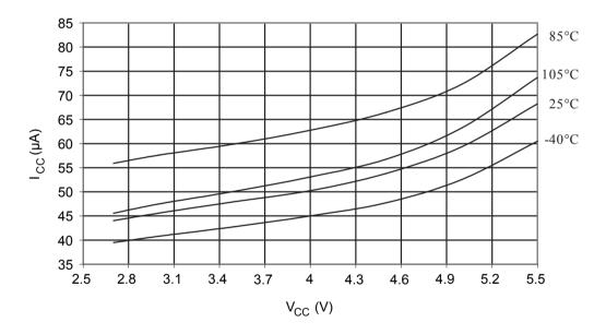
Figure 35-48 Programming Current vs. V<sub>CC</sub>
