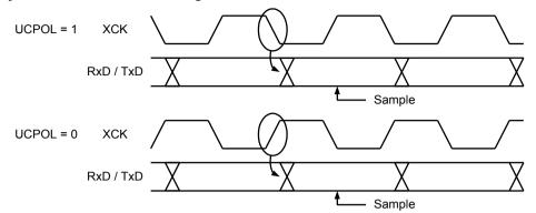
The UCPOL bit UCRSC selects which XCK clock edge is used for data sampling and which is used for data change. As the figure above shows, when UCPOL is zero the data will be changed at rising XCK edge and sampled at falling XCK edge. If UCPOL is set, the data will be changed at falling XCK edge and sampled at rising XCK edge.
