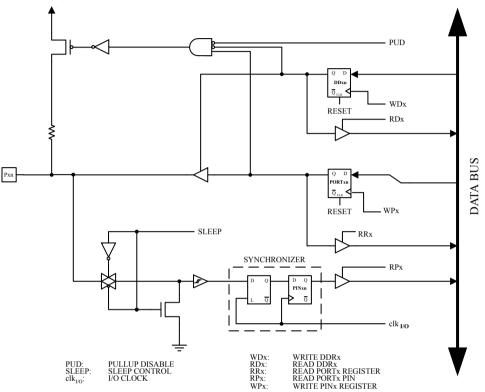
**Note:** 1. WPx, WDx, RRx, RPx, and RDx are common to all pins within the same port.  $clk_{I/O}$ , SLEEP, and PUD are common to all ports
