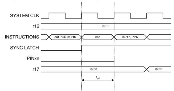
Figure 18-4 Synchronization when Reading a Software Assigned Pin Value
