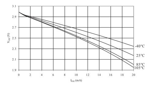
I/O PIN OUTPUT VOLTAGE vs. SOURCE CURRENT NORMAL POWER PINS
