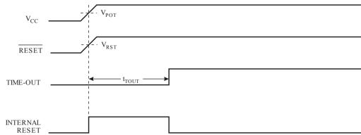
Figure 15-3 Figure: MCU Start-up, RESET Extended Externally
