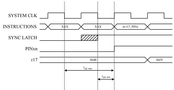
Consider the clock period starting shortly after the first falling edge of the system clock. The latch is closed when the clock is low, and goes transparent when the clock is high, as indicated by the shaded region of the "SYNC LATCH" signal. The signal value is latched when the system clock goes low. It is clocked into the PINxn Register at the succeeding positive clock edge. As indicated by the two arrows
