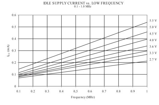
Figure 34-8 Idle Supply Current vs. Frequency (0.1 - 1.0 MHz)
