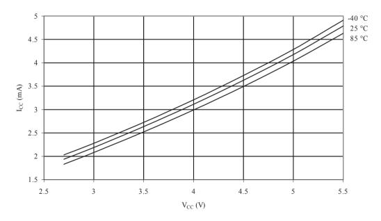
Figure 34-14 Idle Supply Current vs. V<sub>CC</sub> (32 kHz External Oscillator)
