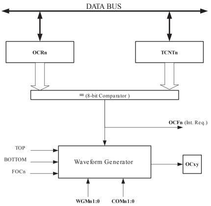
The OCR0 Register is double buffered when using any of the Pulse Width Modulation (PWM) modes. For the normal and Clear Timer on Compare (CTC) modes of operation, the double buffering is disabled. The double buffering synchronizes the update of the OCR0 Compare Register to either top or bottom of the counting sequence. The synchronization prevents the occurrence of odd-length, non-symmetrical PWM pulses, thereby making the output glitch-free.
