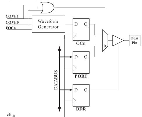
Figure 21-4 Compare Match Output Unit, Schematic
