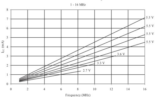
IDLE SUPPLY CURRENT vs. FREQUENCY
