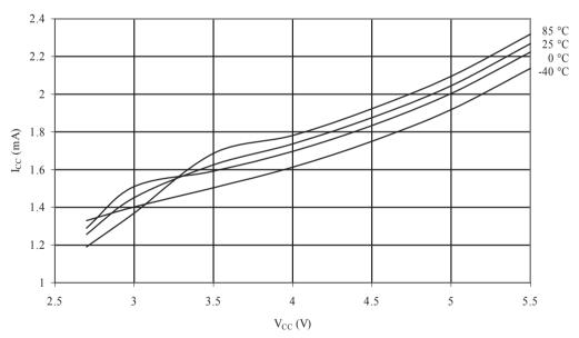
ACTIVE SUPPLY CURRENT vs. V<sub>CC</sub> INTERNAL RC OSCILLATOR. 1 MHz
