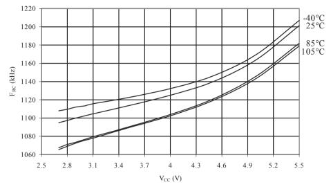
Figure 35-33 Watchdog Oscillator Frequency vs. Temperature
