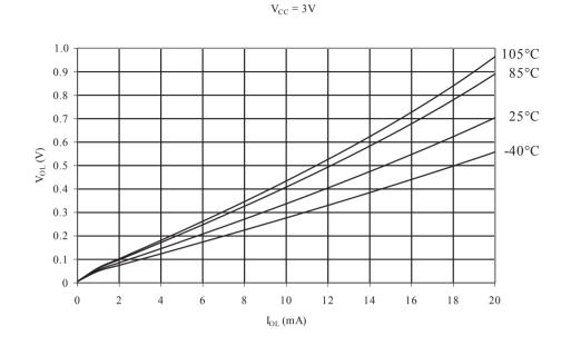
I/O PIN OUTPUT VOLTAGE vs. SINK CURRENT
