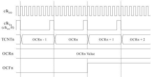
The figure below shows the setting of OCF0 and the clearing of TCNT0 in CTC mode.
