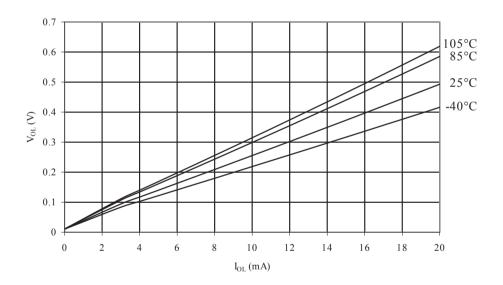
Figure 35-22 I/O Pin Output Voltage vs. Sink Current, Port B (V<sub>CC</sub> = 3V)
