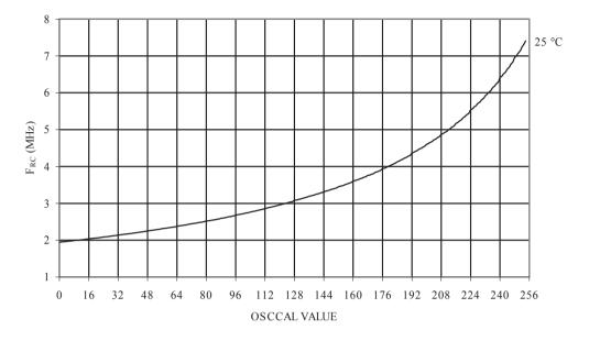
Figure 34-49 Calibrated 8 MHz RC Oscillator Frequency vs. Temperature
