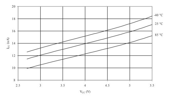
BROWNOUT DETECTOR CURRENT vs. V<sub>CC</sub>
