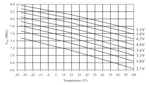
Figure 35-41 Calibrated 8MHz RC Oscillator Frequency vs. V<sub>CC</sub> CALIBRATED 8MHz RC OSCILLATOR FREQUENCY vs. OPERATING VOLTAGE
