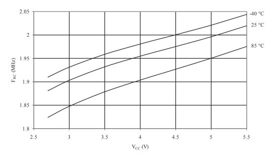
CALIBRATED 2MHz RC OSCILLATOR FREQUENCY vs. Vcc
