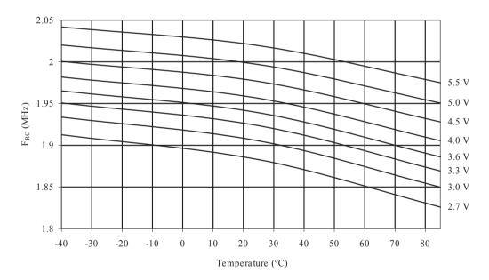
Figure 34-44 Calibrated 2 MHz RC Oscillator Frequency vs. V<sub>CC</sub>
