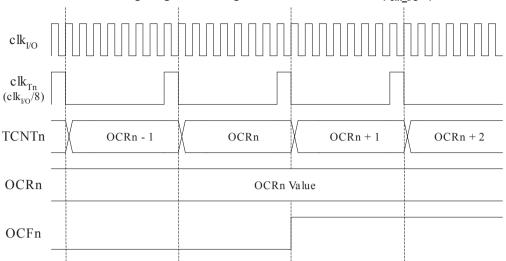
The next figure shows the setting of OCF2 and the clearing of TCNT2 in CTC mode.
