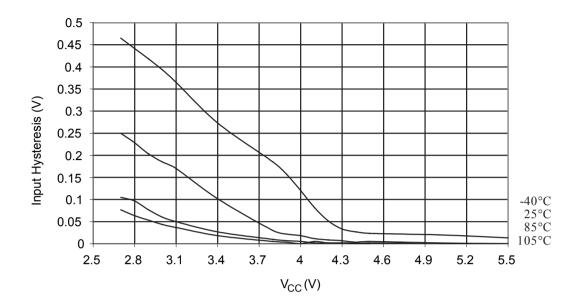
Reset Input Pin Hysteresis vs. V<sub>CC</sub>
