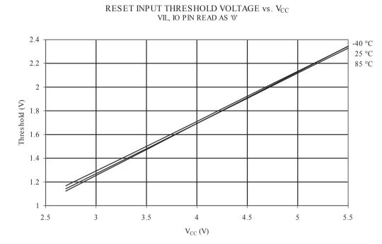
Figure 34-35 Reset Input Pin Hysteresis vs. V<sub>CC</sub>
