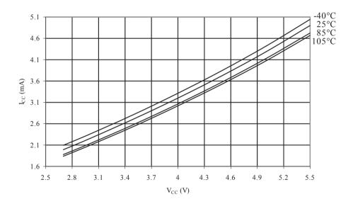
Figure 35-10 Idle Supply Current vs. V<sub>CC</sub> (Internal RC Oscillator, 4MHz)
