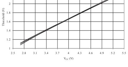
Figure 35-25 I/O Pin Input Hysteresis vs. V<sub>CC</sub>
