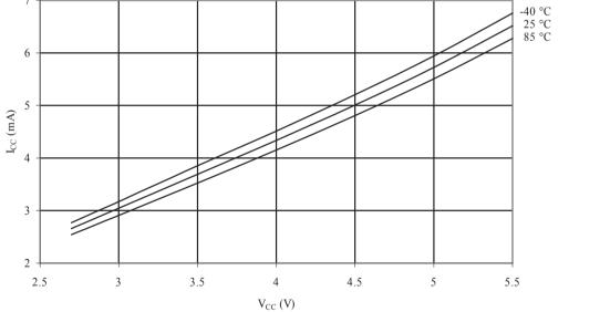
Figure 34-6 Active Supply Current vs. V<sub>CC</sub> (Internal RC Oscillator, 8 MHz)
