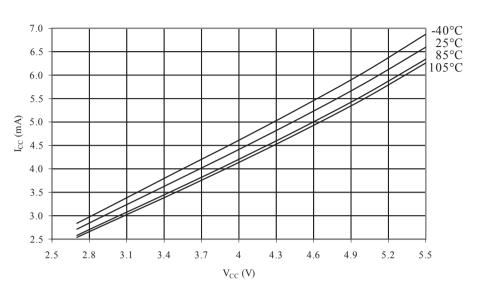
ACTIVE SUPPLY CURRENT vs.  $V_{CC}$  internal RC oscillator, 4 MHz
