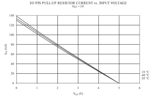
Figure 34-20 I/O Pin Pull-up Resistor Current vs. Input Voltage (V<sub>CC</sub> = 5V) I/O PIN PULL-UP RESISTOR CURRENT vs. INPUT VOLTAG
