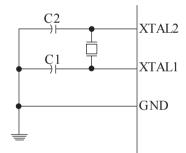
The Oscillator can operate in three different modes, each optimized for a specific frequency range. The operating mode is selected by the fuses CKSEL3:1 as shown in the following table.
