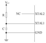
The Oscillator can operate in four different modes, each optimized for a specific frequency range. The operating mode is selected by the fuses CKSEL3:0 as shown in the following table.
