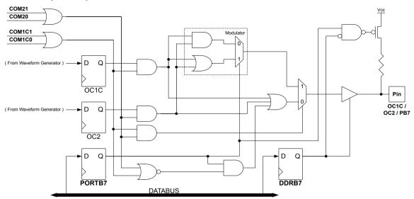
When the modulator is enabled the type of modulation (logical AND or OR) can be selected by the PORTB7 Register. Note that the DDRB7 controls the direction of the port independent of the COMnx1:0 bit setting.
