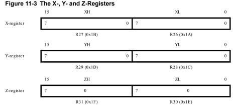
In the different addressing modes these address registers have functions as fixed displacement, automatic increment, and automatic decrement (see the Instruction Set Reference for details).
