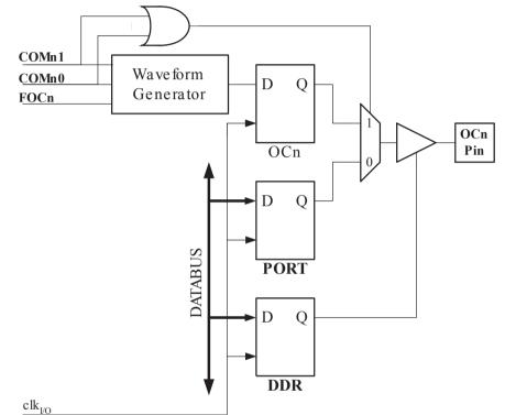
The general I/O port function is overridden by the Output Compare (OC2) from the waveform generator if either of the COM21:0 bits are set. However, the OC2 pin direction (input or output) is still controlled by the Data Direction Register (DDR) for the port pin. The Data Direction Register bit for the OC2 pin (DDR\_OC2) must be set as output before the OC2 value is visible on the pin. The port override function is independent of the Waveform Generation mode.
