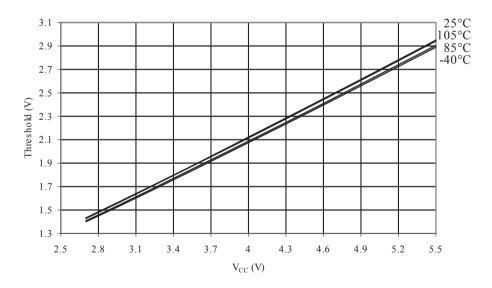
I/O P IN INPUT THRESHOLD VOLTAGE vs.  $V_{\rm CC}$ VIL, IO PIN READ AS '0' 105°C 85°C 25°C -40°C 2.4 2.2 2 Threshold (V) 1.8 1.6 1.4 1.2 1 2.5 2.8 3.1 3.4 3.7 4 4.3 4.9 5.2 5.5 4.6
