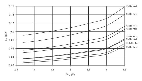
STANDBY SUPPLY CURRENT vs. V<sub>CC</sub>
