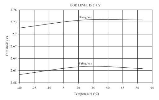
BOD THRESHOLDS vs. TEMPERATURE
