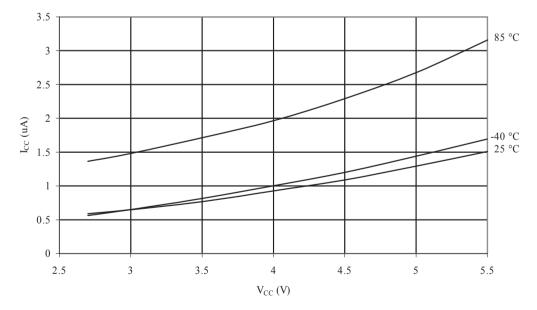
Figure 34-16 Power-Down Supply Current vs. VCC (Watchdog Timer Enabled)
