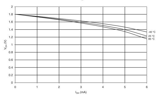
Figure 19-34.  $V_{OH}$ : I/O Pin Output Voltage vs. Source Current ( $V_{CC} = 3V$ )
