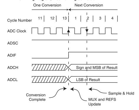
Figure 14-7. ADC Timing Diagram, Free Running Conversion
