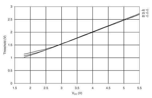
Figure 19-49.  $V_{IL}$ : Input Threshold Voltage vs.  $V_{CC}$  (Reset Pin as I/O, Read as '0')
