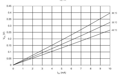
Figure 19-38.  $V_{OL}$ : I/O Pin Output Voltage vs. Sink Current ( $V_{CC} = 5V$ )
