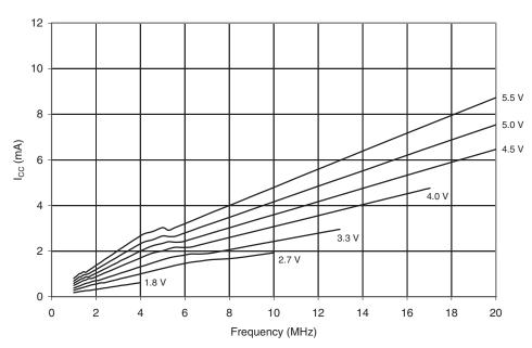
Figure 19-3. Active Supply Current vs.  $V_{CC}$  (Internal RC Oscillator, 9.6 MHz)
