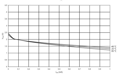
Figure 19-41.  $V_{OH}$ : Reset Pin as I/O, Output Voltage vs. Source Current ( $V_{CC} = 5V$ )
