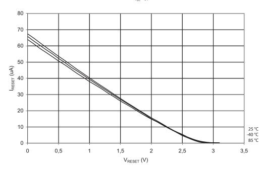
Figure 19-26. Reset Pull-up Resistor Current vs. Reset Pin Voltage ( $V_{CC} = 5V$ )
