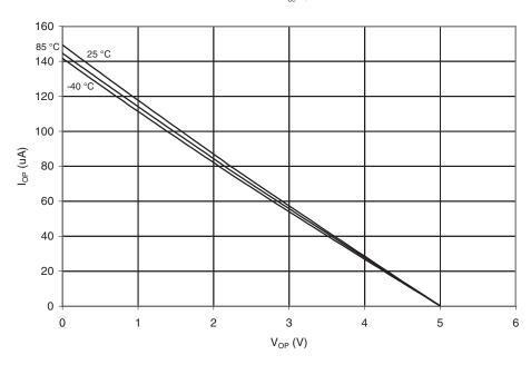
Figure 19-24. Reset Pull-up Resistor Current vs. Reset Pin Voltage ( $V_{CC} = 1.8V$ )
