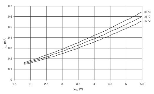
Figure 19-11. Idle Supply Current vs.  $V_{\rm CC}$  (Internal RC Oscillator, 128 kHz)
