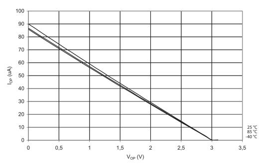
Figure 19-23. Pull-up Resistor Current vs. Input Voltage (I/O Pin,  $V_{CC} = 5V$ )
