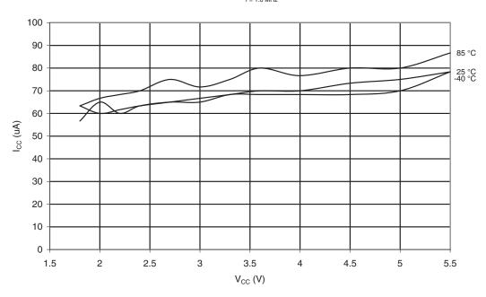
Figure 19-20. Programming Current vs. V<sub>CC</sub>
