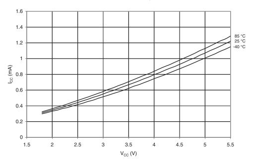
Figure 19-10. Idle Supply Current vs.  $V_{\rm CC}$  (Internal RC Oscillator, 4.8 MHz)
