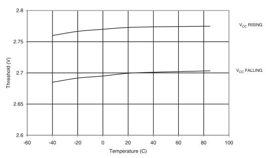
Figure 19-53. BOD Thresholds vs. Temperature (BODLEVEL is 1.8V)
