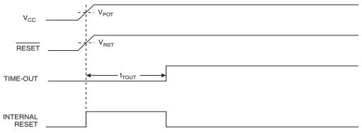
Figure 8-3. MCU Start-up, RESET Extended Externally
