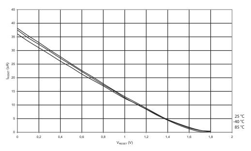
Figure 19-25. Reset Pull-up Resistor Current vs. Reset Pin Voltage ( $V_{CC} = 3V$ )
