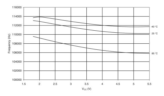
Figure 19-66. 128 kHz Watchdog Oscillator Frequency vs. Temperature
