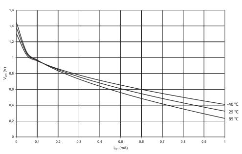
Figure 19-40.  $V_{OH}$ : Reset Pin as I/O, Output Voltage vs. Source Current ( $V_{CC} = 3V$ )
