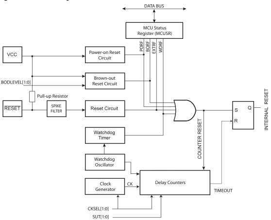
The I/O ports of the AVR are immediately reset to their initial state when a reset source goes active. This does not require any clock source to be running.
