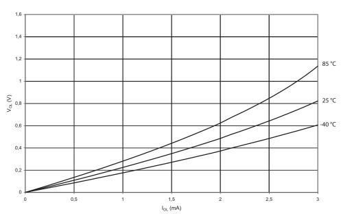
Figure 19-44.  $V_{OL}$ : Reset Pin as I/O, Output Voltage vs. Sink Current ( $V_{CC} = 5V$ )
